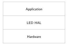
The LED HAL is implemented in the led.c and led.h files.
